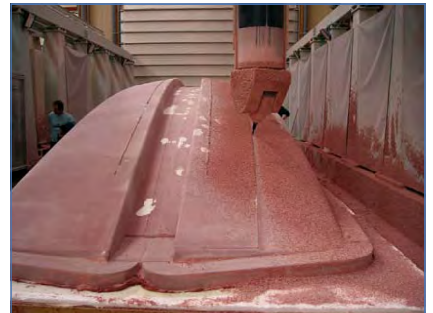
5 Axis machining of the X-35 Hull Plug
